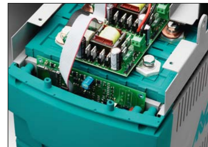
Top: The Mastervolt factory outside Amsterdam, Holland. Left: Detail showing PCBs buried beneath the surface of the battery. Above: The handles fold flat.
