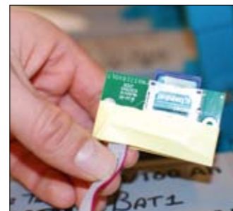
Right: Every battery undergoes a rigorous automated test procedure. Top: Among the electronics that control the individual cells is an SD card for recording battery use. Above: Detail of SD card.
