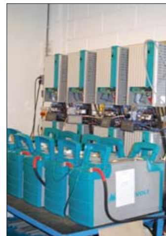
Right: Every battery undergoes a rigorous automated test procedure. Top: Among the electronics that control the individual cells is an SD card for recording battery use. Above: Detail of SD card.
